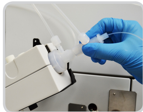
Correct method for removing the C-Flow from the spray chamber end cap. Grasp the nebulizer body only, and not the uptake line.
