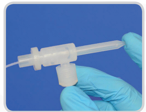
Clearing air gaps in an uptake line by backflushing.
