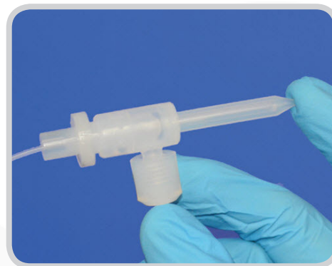
Clearing air gaps in an uptake line by backflushing.
