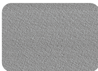
Purillex PFA Bottle Inside Base (1000x SEM Magnification)
