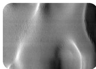
Competitor PFA Bottle Inside Base (1000x SEM Magnification)
