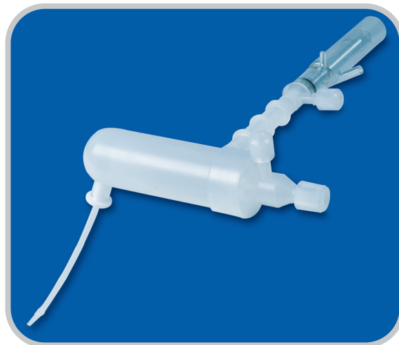
PFA Inert Sample Introduction Kit Compatible with Agilent ICP-MS
