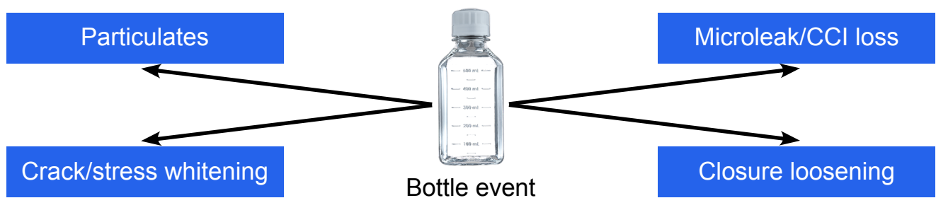
Figure 5. Common container failure pathways after sterilization
