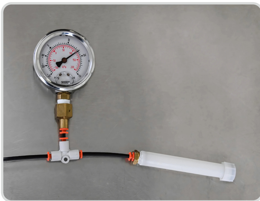
Pressurized integrity testing of Purillex containers
