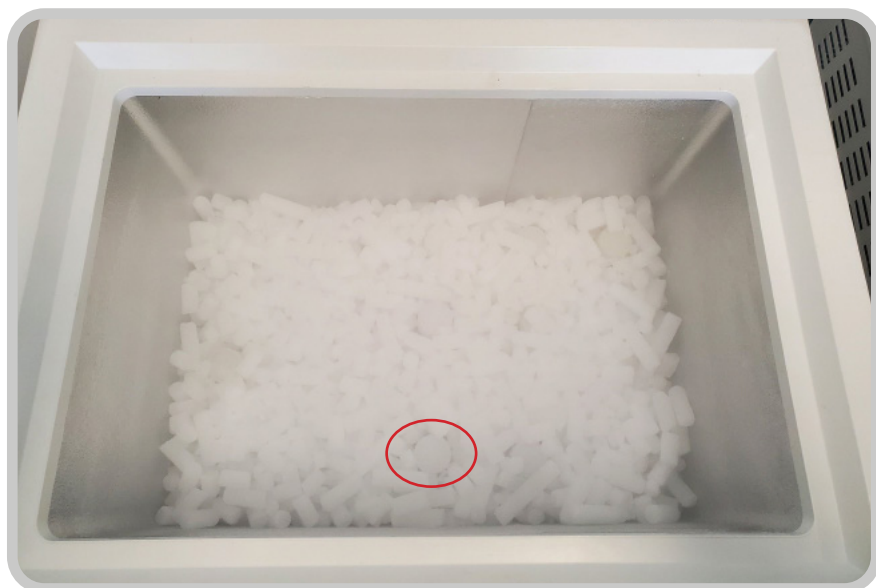
Figure 2: 1L Purillex PETG Bottles packed in dry ice (note that only bottle closures can be seen in the image)
