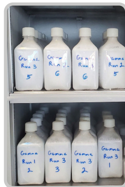
Figure 1: 1L Purillex PETG Bottles in upright freezer at -85°C (control bottles)
