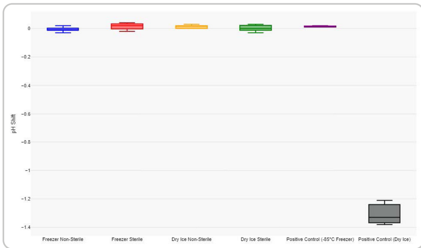
Figure 3: pH Shift in Saville Purillex PETG Bottles after freezing in dry ice and conventional freezer
