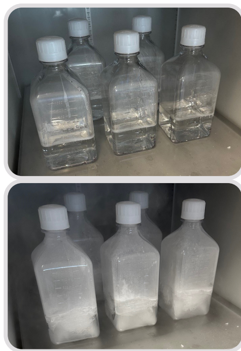
Figure 2: Bottles in -85^{\circ}\text{C} upright freezer, before and after freezing (for illustrative purposes only)
