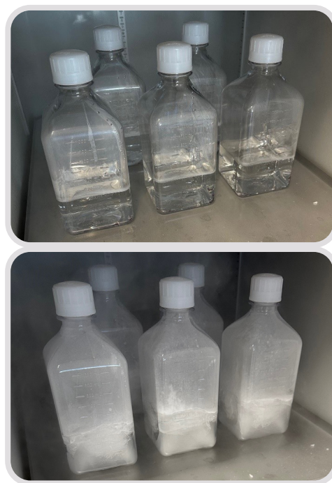
Figure 2: Bottles in -85°C upright freezer, before and after freezing (for illustrative purposes only)
