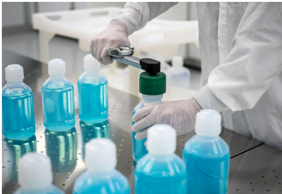
Precise closure torque is key to maintaining container integrity
