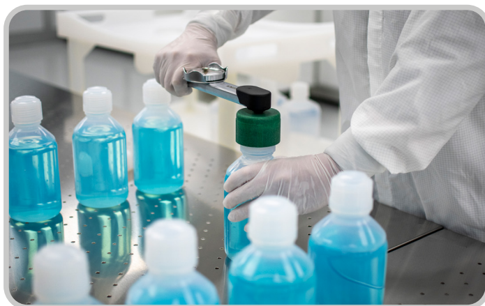
Precise closure torque is key to maintaining container integrity
