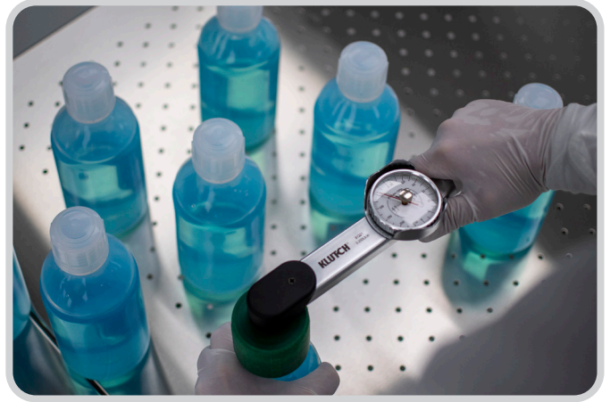
Torque being applied to bottle closures using torque wrench with closure adaptor
