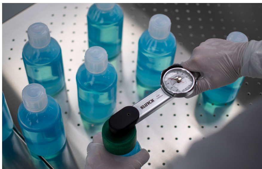
Torque being applied to bottle closures using torque wrench with closure adaptor
