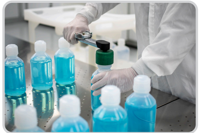
Precise closure torque is key to maintaining container integrity
