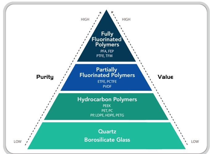
Figure 1: Fluoropolymers are innately higher in purity, and due to improved performance, higher in value than common hydrocarbon plastics like PE and PP
