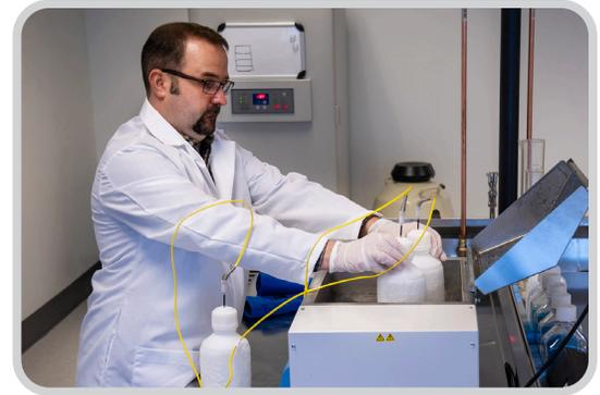
*Placing bottles in 37°C preheated recirculating water bath*
