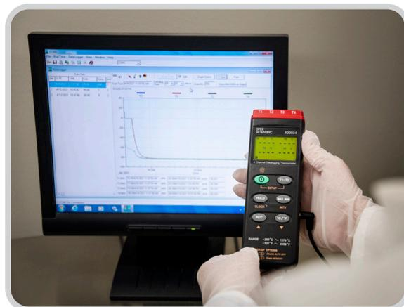
*Uploading recorded data from 4-channel datalogger with Type K thermocouples*
