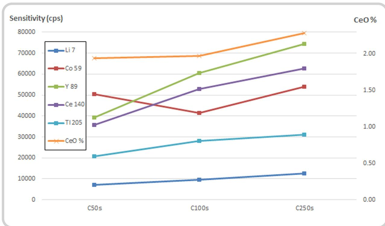
Figure 1. Sensitivity comparison for C50s, C100s and C200s. Orange line (with cross marks) is CeO ratio (right side axis).
